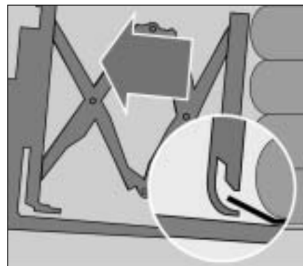
6. Retract the pusher plate. The gripper bar will automatically clamp the slipsheet lip.
