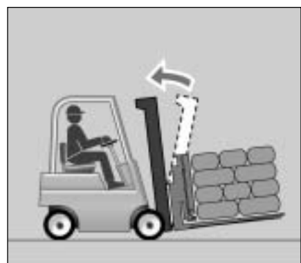
9. Tilt the mast back, and raise the load three-to-four inches above the floor. You are now ready to transport the load.
