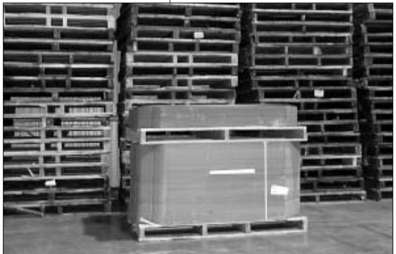
Photo shows hundreds of slipsheets stored on pallet, providing sharp contrast to wooden pallet storage.
