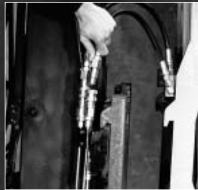
2. Connect quick-change hydraulic couplers
