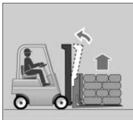
8. As the weight of the load is transferred to the platens, they will deflect downward slightly. Raise the carriage about one inch to prevent the platen from digging into the floor. Slowly tilt the mast to a vertical position as you scoop up the load.
